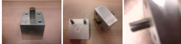
Figure A- 1: Gold Stamp. The gold stamp consists of two machined aluminum blocks and a serrated carbide plunger. The sample is placed gold side up between the two aluminum blocks and the serrated tip is used to impress lines onto the gold surface. Subsequently turning the upper block 90 degrees and impressing a second set of lines will create a grid.
